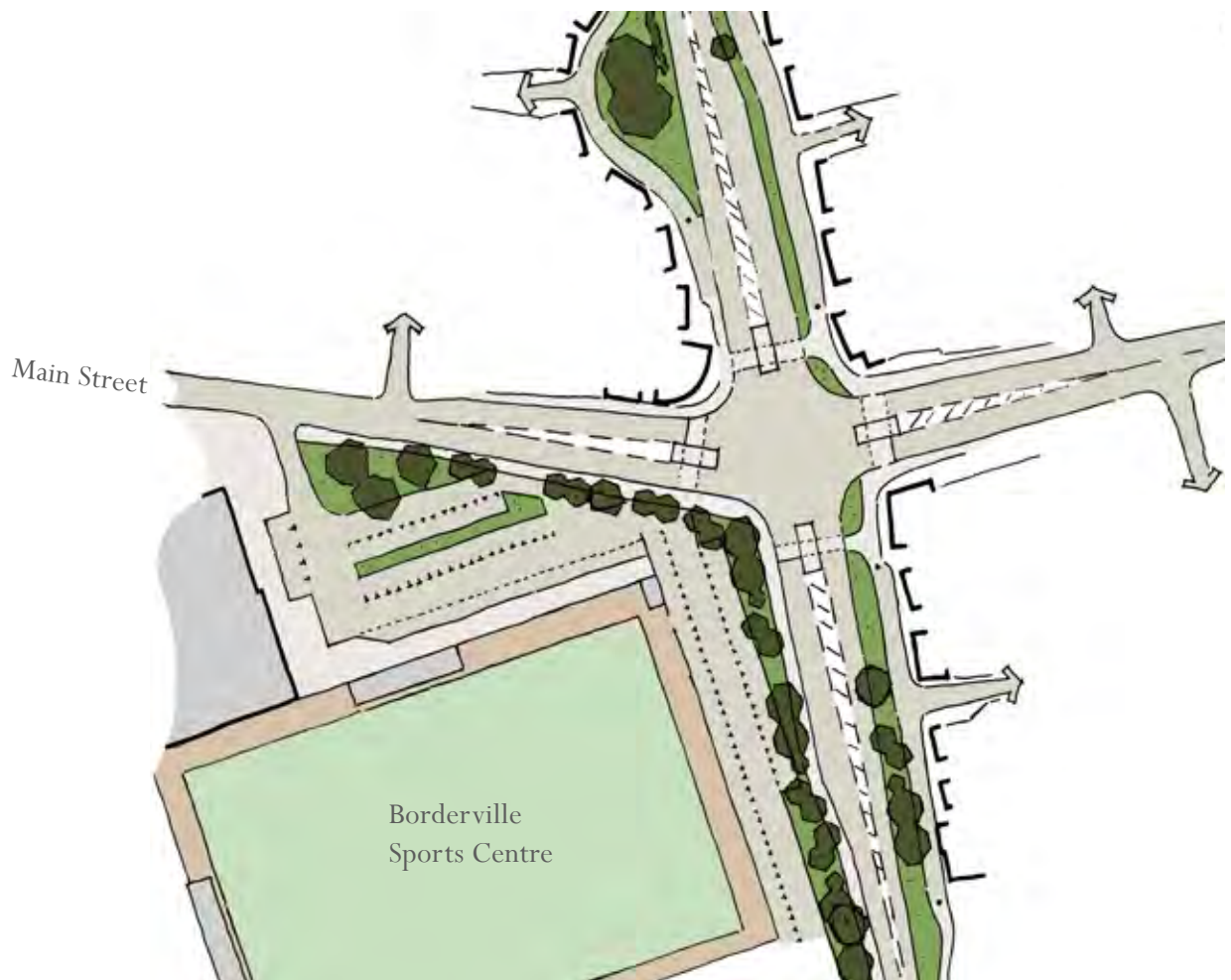
Fig 56. Potential arrangement of junction with Ryhall Road. The choice of junction form at this location has been determined by the requirements for forward visibility from the north.
